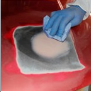
1 Clean and inspect repair area.
